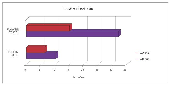
Flowtin TC300 with micro additives reduces the dissolution rate of copper wires und therefore decreases the reduction of the diameter of the copper wire. If dross may be an issue on static solder bath, it may be advantageous to add on a regular base lead-free Anti-Oxidation-Pellets. This keeps the surface of the solder bath clean and free of dross.
